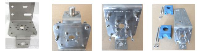
Install the 4 bolts 4x25MA (for wire radials) in the holes in X shape (inner bolts are used only in the solid radials version). On one of those will take place one end of the RF choke eyelet terminal. Correct assembling sequence for all the bolts: bolt, serrated washer, normal nut, two flat washers and self-locking nut.
