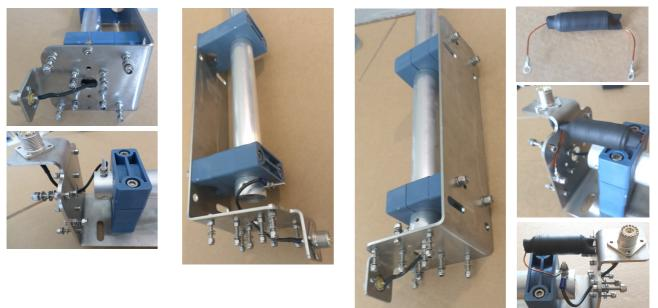
With the aid of the U bolts, install the base on the supporting pole and install the wire radials. The U bolts are 50mm wide, it can get poles or tubes from 40 to 50mm.
